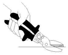
Offset snips permit you to keep your hands safely above the cut while cutting directly through the centre of a large sheet.
